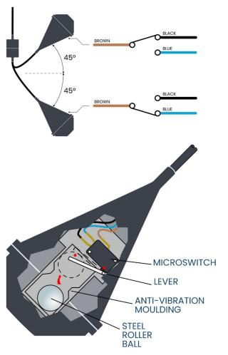
**NOTE:** If tethering is required, do not secure the float switch too close to the float body, as this may impede correct operation.
